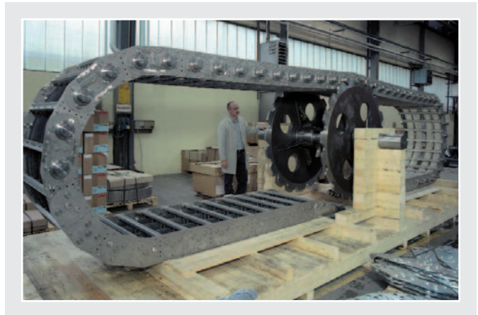
Steel cable carrier with load-bearing bolts.
