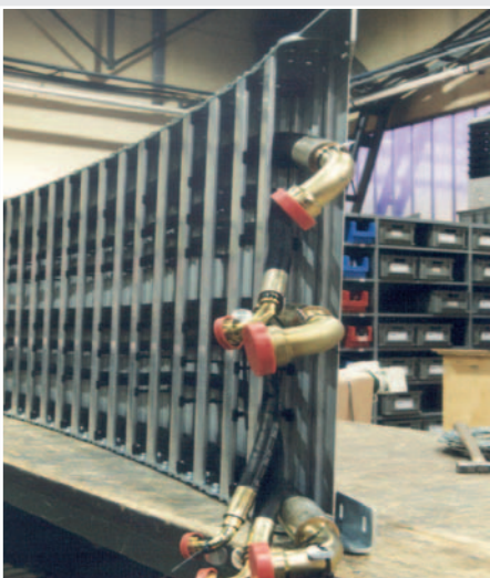
Steel cable carriers with hydraulic hoses.
