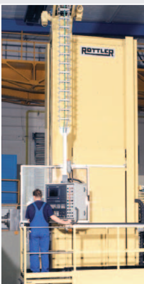
Steel cable carriers with load-bearing bolts. Photograph: Rottler GmbH
