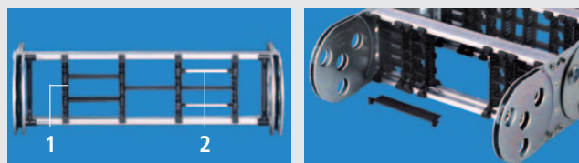
Vertical separations with dividers (1) Horizontal height separations with partitions made of plastic or aluminium (2). These can also be installed at a later date or modified by changing the partitions.
