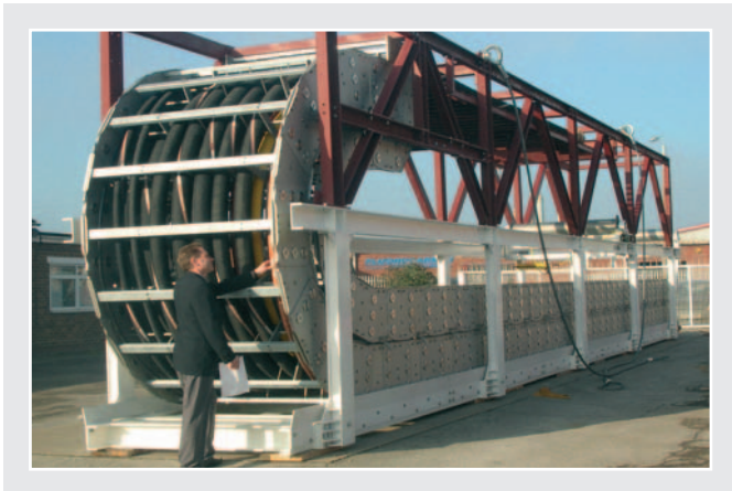
Steel cable carriers on transport frame.
