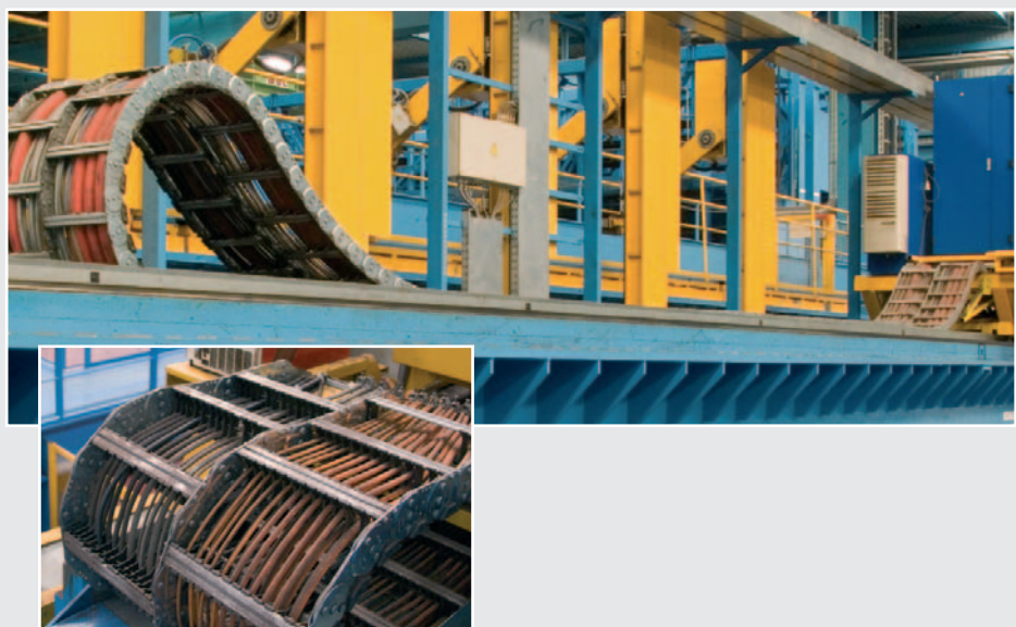
Steel cable carriers on a laser cutting machine. Photographs: Meyer Werft GmbH
