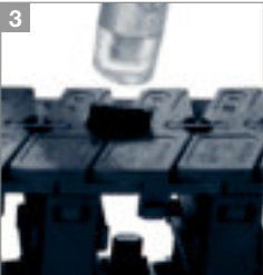
3 Gently reinsert connector by using hammer
