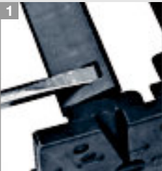
1 Lever crossbars with screwdriver
