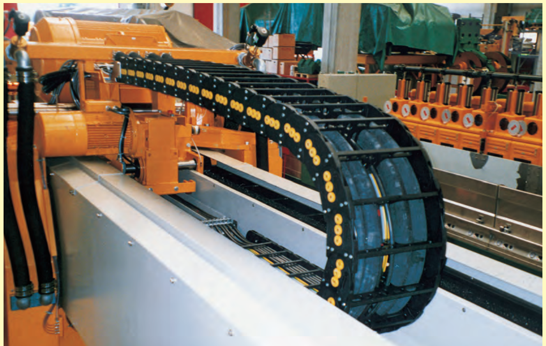
Nylon chain, type 310, in a self-supporting state.
