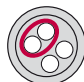
Element shield continuous bending hi-flex, tin-plated braided copper shield with the option of foil shield – see type/design
