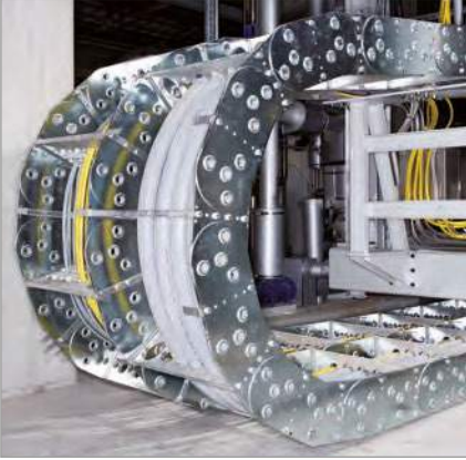
Steel cable carriers on a paper machine Photographs: Voith Paper Technology Center GmbH
