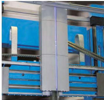
■ Telescopic cover at a milling machine
