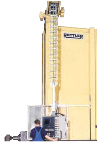
Steel cable carriers on a CNC drilling machine Photographs: Rottler Rottler Werkzeugmaschinen GmbH
