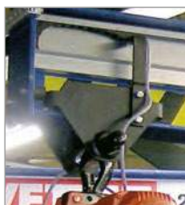
MONO cable carriers on a pillar jib crane
