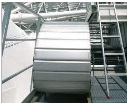
Steel cable carriers on a scissored coil lift Photographs: SÜDO GmbH
