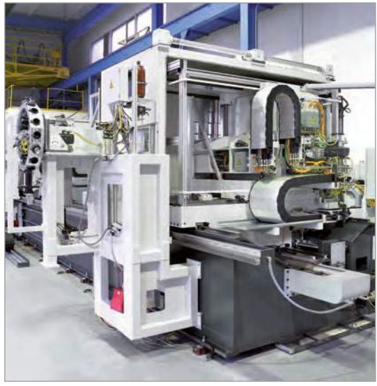
Cable and hose carriers of the MASTER LT series on a tube end processing machine Photographs: Rottler Werkzeugmaschinen GmbH
