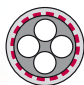
Overall shield continuous bending hi-flex, tin-plated copper braiding for smallest bend radii
