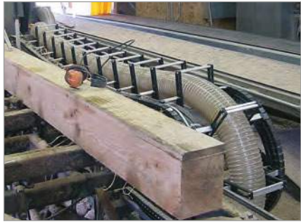
QUANTUM cable carrier system on a wood processing machine
