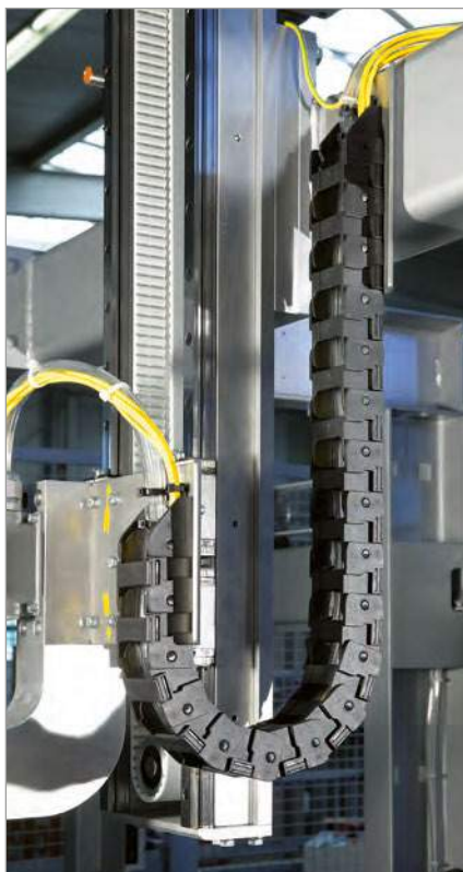
MONO and UNIFLEX Series cable carriers in packaging machines
