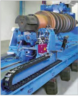
Cable and hose carriers of the UNIFLEX and MONO series on a roll neck milling machine Photographs: Rottler Werkzeugmaschinen GmbH
