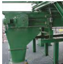
■ Scraper conveyor for distribution of various chip materials
