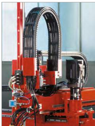
QUANTUM cable carrier system on a handling system
