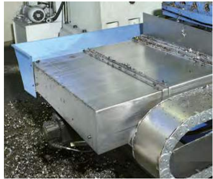
■ Telescopic cover at a milling machine
