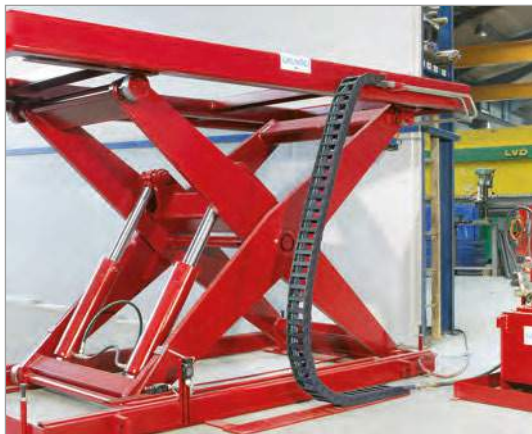
UNIFLEX Series cable and hose carriers on a scissored coil lift Photographs: Grunδει Hebetische Verladetechnik GmbH
