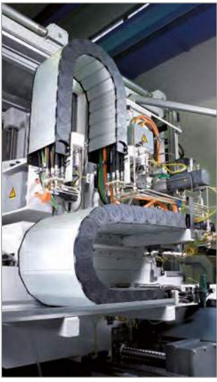
Cable and hose carriers of the MASTER LT series on a tube end processing machine Photographs: Rottler Werkzeugmaschinen GmbH
