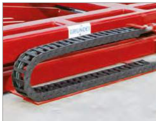
UNIFLEX Series cable and hose carriers on a scissored coil lift Photographs: Grunδει Hebetische Verladetechnik GmbH
