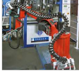
ROBOTRAX cable carrier system: Angle of rotation about 180° without channel system on a buckling arm robot application Photographs: Reis Robotics, Arthur Bräuer GmbH & Co. KG
