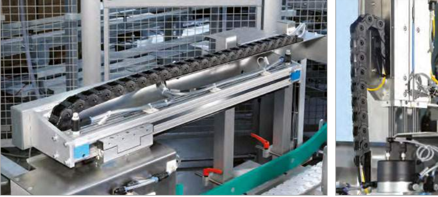
UNIFLEX Series cable carrier on a packaging machine Photographs: Transnova-Ruf GmbH
