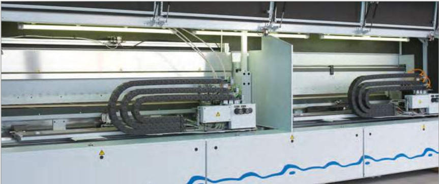
UNIFLEX Series cable and hose carriers on an automatic wood processing machine Photographs: Homag Holzbearbeitungssysteme AG
