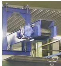
■ Hinged belt conveyor for loading of a hopper system
