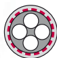
Overall shield high flexural strength, tin-plated copper braiding for small bend radii
