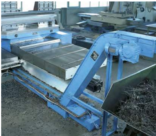
■ Standard hinged belt conveyor at a CNC boring machine
