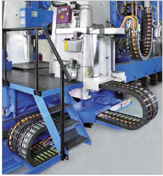
Cable and hose carriers of the UNIFLEX and MONO series on a roll neck milling machine Photographs: Rottler Werkzeugmaschinen GmbH
