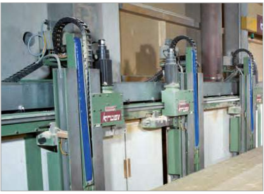
MONO Series cable and hose carriers on a wood processing machine Photographs: Krüsi Maschinenbau AG
