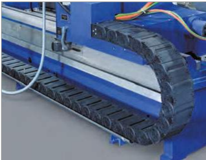
Type MT 0950 cable carrier on a roll grinding machine Installation variant: horizontal – "unsupported"
