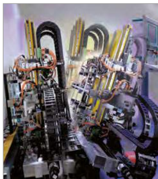
UNIFLEX Series cable carriers on an automatic window frame setting station Photographs: Lenhard Maschinenbau GmbH
