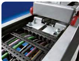
Automatic emergency cut-off with decoupling of the cable carrier
