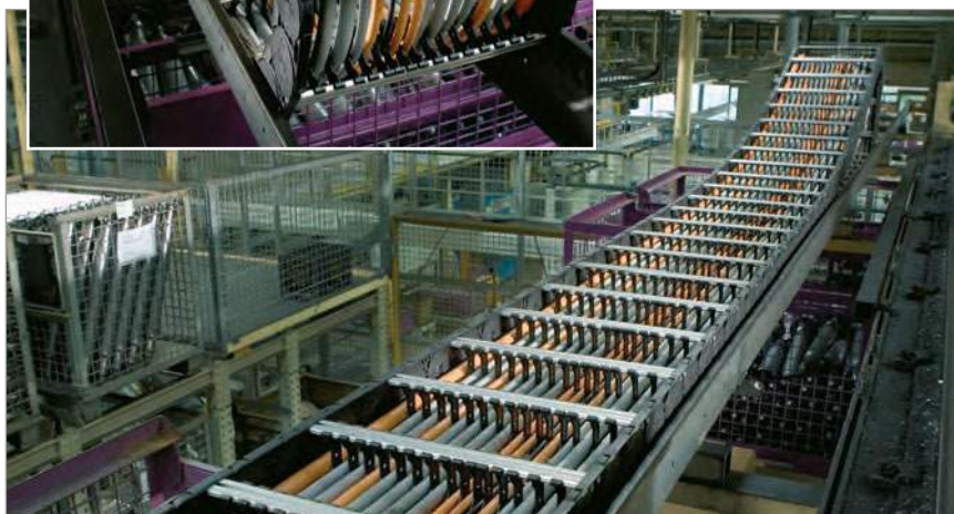
M Series cable and hose carriers on a highrise rack Photographs: BMW AG
