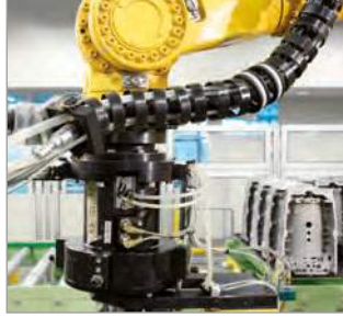
ROBOTRAX cable carriers on a jointed-arm robot Photographs: Daimler Chrysler AG
