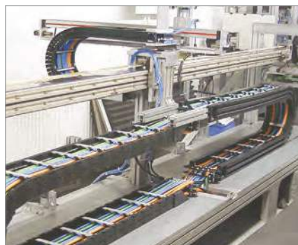
■ High-speed test stand ■ Durability tests exceeding 25 million cycles
