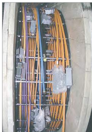
■ 125 m travel length: carrier fully harnessed with TRAXLINE Series 700
