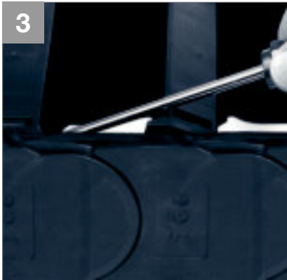
3 Assemble crossbars - push down and snap in by using a screwdriver
