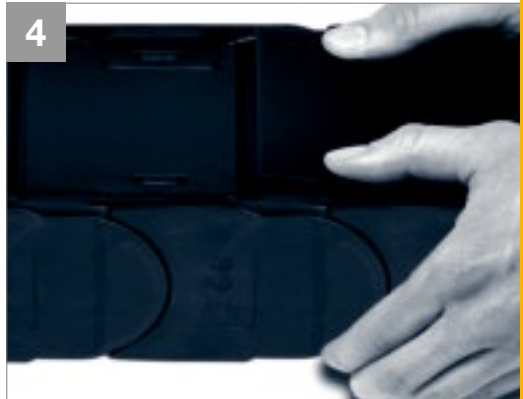
4 e-tube: assemble lids/bottoms - attach to the connector at an angle - snap in
