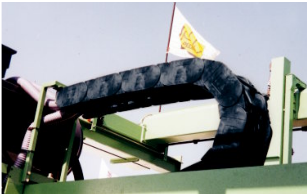
Unsupported, harnessed Series 1640 in a stone machining application
